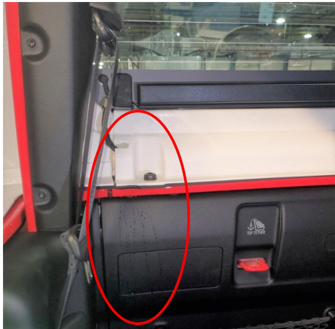
Fig. 1 Water Leak At Backlite
