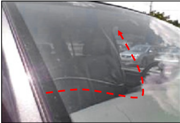
Single crack with no impact mark: Warranty
