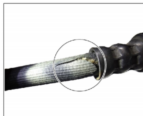
Example of crack in brake hose
