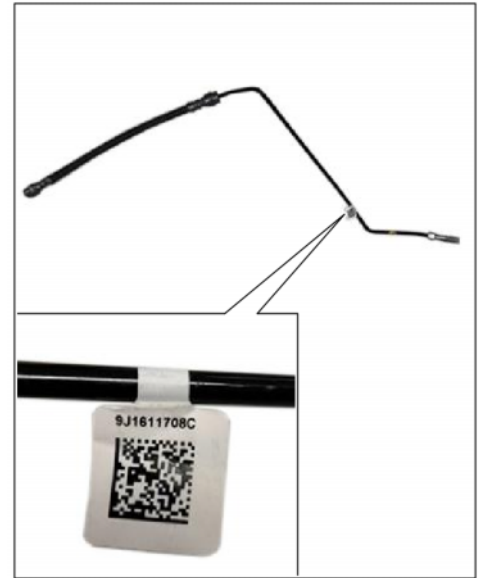
Label on damaged brake hose
