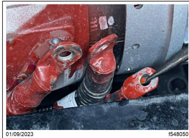
Fig. 2, Corrosion Sealer Applied on the Ground Cable Mounting Eyes
