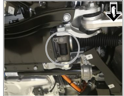
Rubber-metal mount (shown on the right side of the vehicle)
