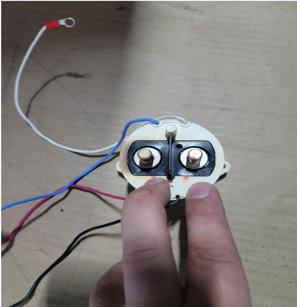
Fig 3: +A1 and A2- markings on the contactor terminals
