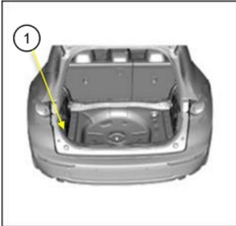
(1) Location of Trunk side insulator
