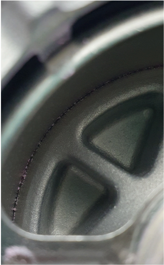
Using Light Source to Detect Debris.png
