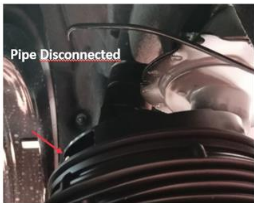
Sample of incorrect Air Suspension pipe installation on the Rear Air Spring
