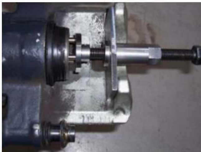
Figure 5: stuck brake calipers piston and sample tool to push it back.
