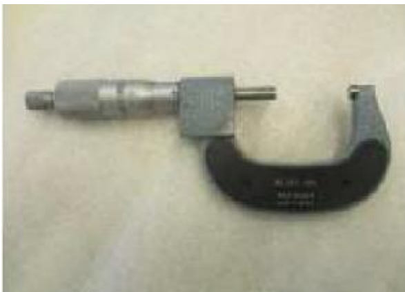
Figure 1: example of micrometer to be used for the measures (left) and measurement points on the brake disc (right).
