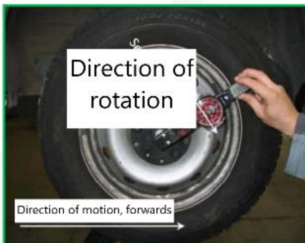
Figure 2: residual braking torque check.
