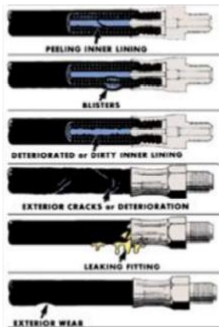
Figure 7: possible hose problems. From top to bottom: inner lining peeling, blister, deteriorated or dirty inner lining, exterior cracks or deterioration, leaking fitting, exterior wear.
