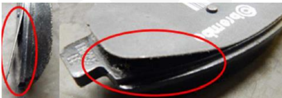
Figure 8: metallic anti-vibration shims detachment from the brake pad.
