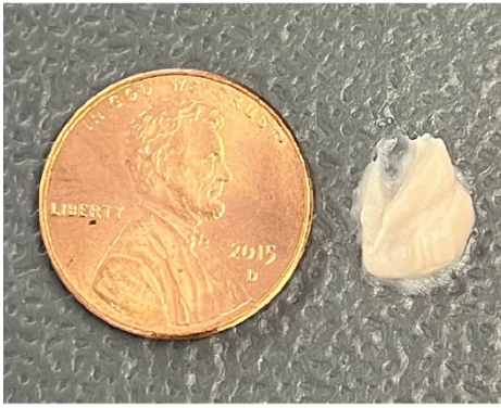
Penny used as a size reference to show the amount of grease used.
