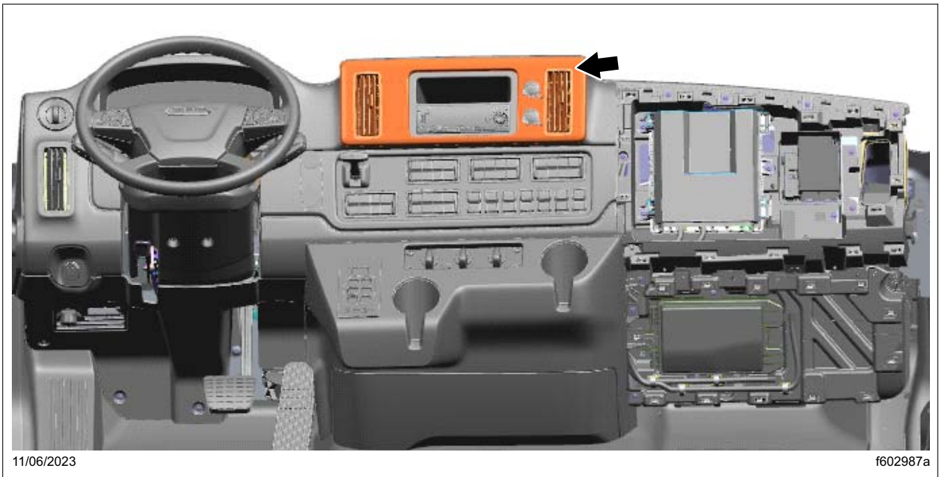
Fig. 8, Upper-Center Fascia Panel
