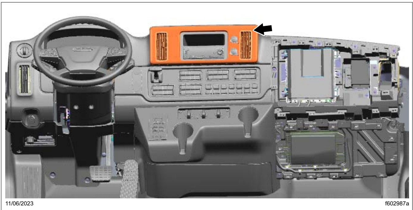
Fig. 2, Upper-Center Fascia Panel
