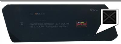
Turn the ignition on and confirm that the connected vehicle reception strength icon shows "X"
