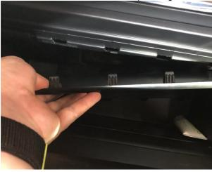
b. Loosen the passenger side airbag mounts.
