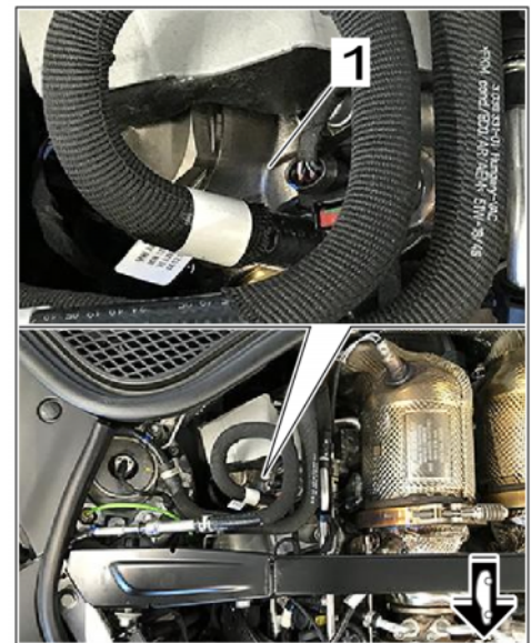
Contact point on high-pressure pump
