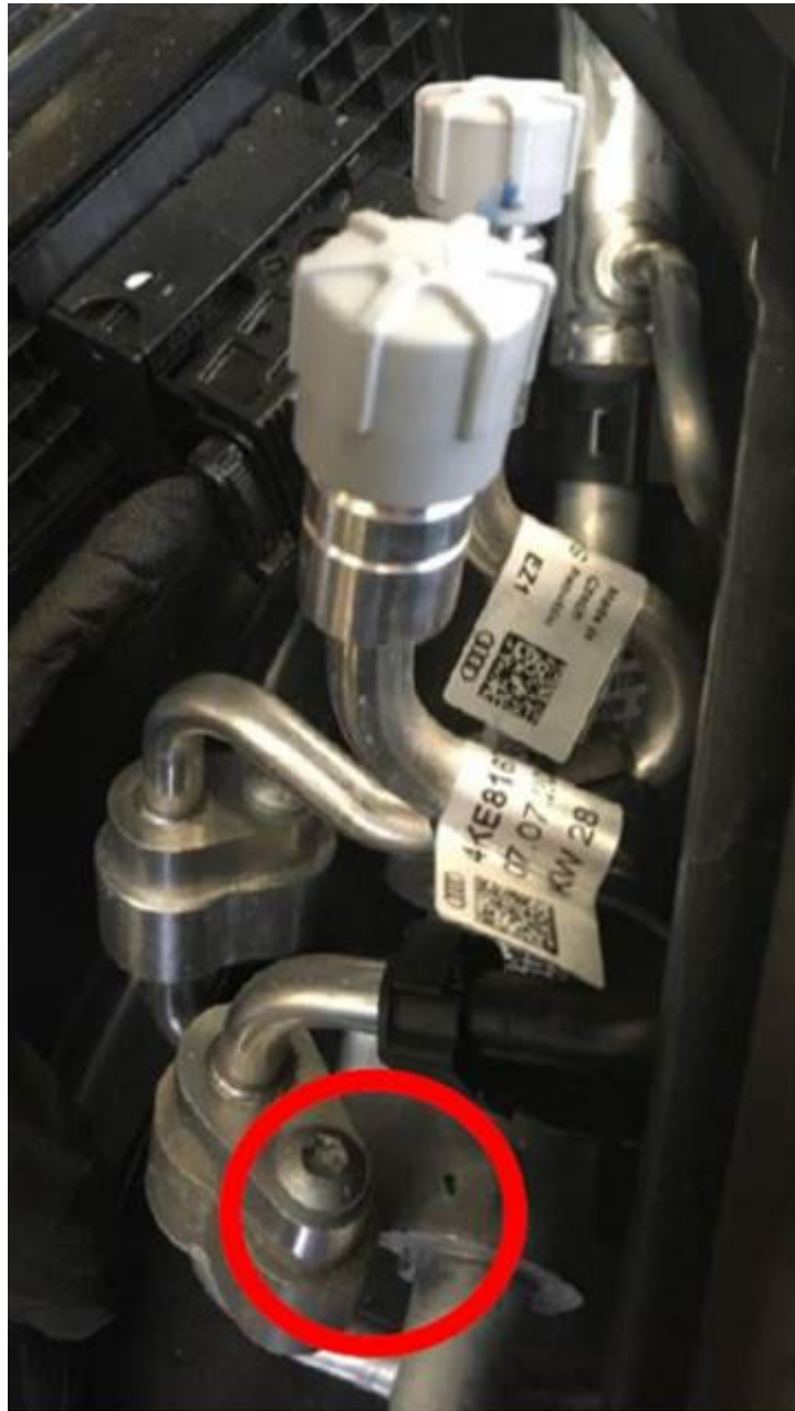
Figure 3. The refrigerant lines are making contact.
