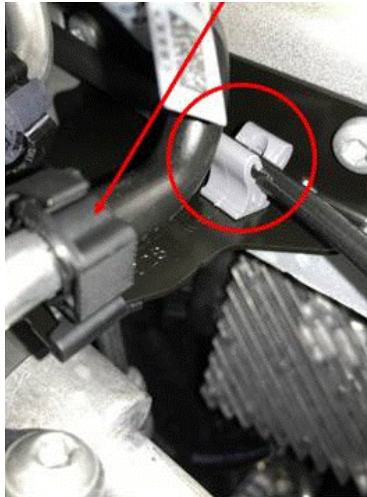
Figure 7. Point of contact between refrigerant line and Bowden cable clip.
