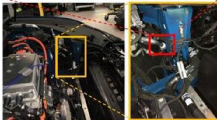
Figure 5. The area in the motor bay where contacting lines are located.
