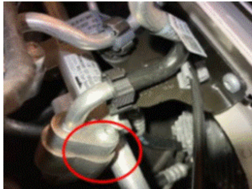
Figure 11. Service port mounting interference with adjacent line.
