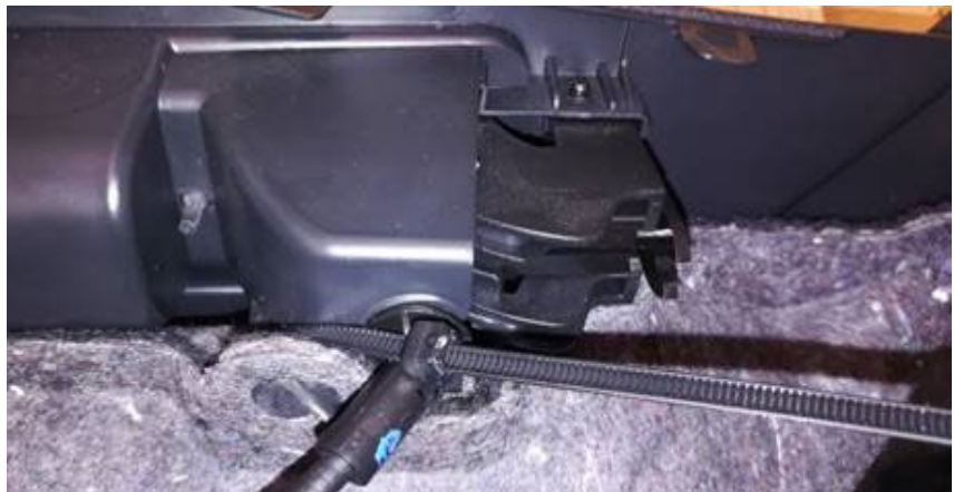
Figure 2. The Bowden cable; reinstalled and secured with a tie wrap.
