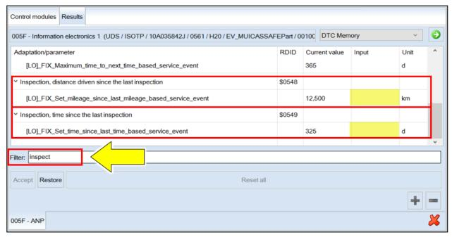
TIP: Enter "inspect" in the Filter field <arrow> and both adaptation channels will be shown.
