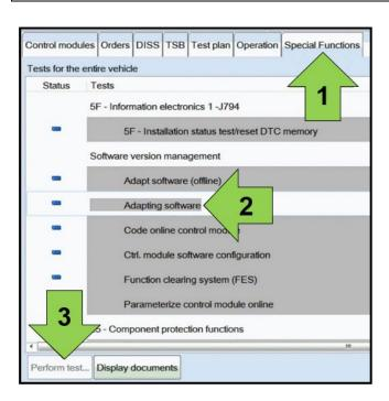
Once the GFF scan is complete, select "Special functions" <arrow 1>, then "Adapting software" <arrow 2>, then select "Perform test" <arrow 3>.
