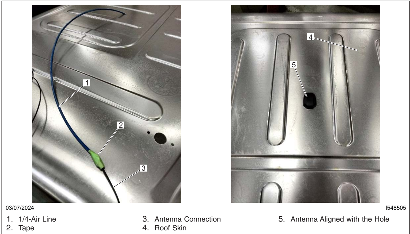
Fig. 9, Aligning the Antenna with the Holes
