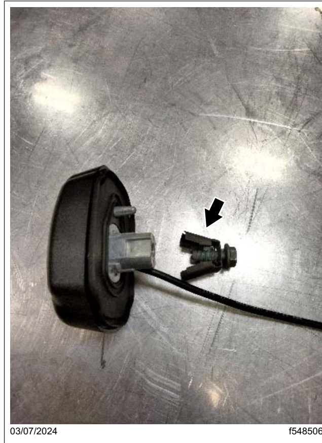
Fig. 10, Antenna Clamp and Bolt Removed
