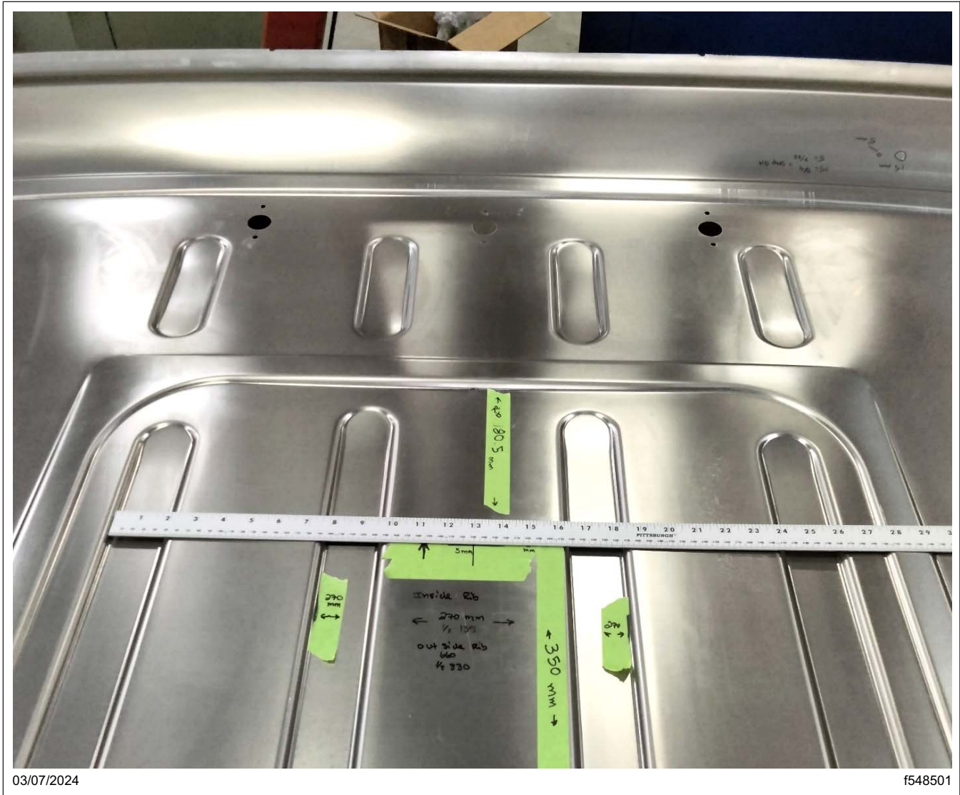
Fig. 5, Marking the Drill Locations on the Roof Skin
