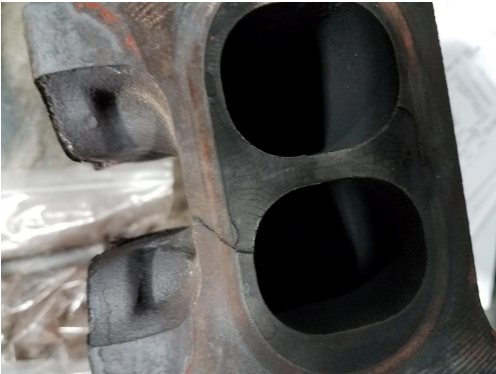
Cracks in the manifold or warped face causing leaks at gasket
