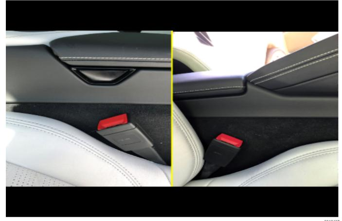
4. Reinstall the front floor rear console side trim panels, assuring no part of the tie-strap is visible. Refer to *Front Floor Rear Console Side Trim Panel Replacement - Left Side and Right Side* in SI.
