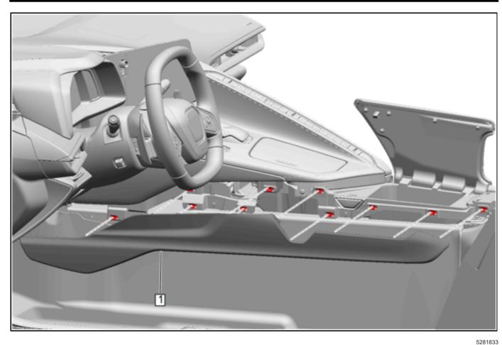
1. Remove the front floor rear console side trim panels (1). Refer to *Front Floor Rear Console Side Trim Panel Replacement - Left Side and Right Side* in SI.
