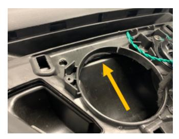
2. Apply a felt strip (50 mm length / 10 mm width) between the center speaker holder and the air duct.
