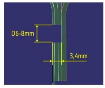
5. Using a weld spot drill bit, drill a hole with a diameter of 6-8 mm through the first three sheet metal layers.
