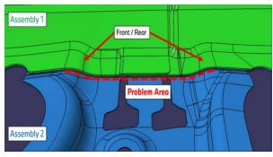
Movement of the sheet metal layers at the B-pillar(s).
