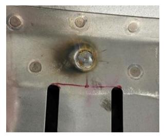
7. To ensure proper welding connection, the paint and corrosion protection around the drilled hole must be carefully sanded off. Seal the hole using MIG/MAG (metal inert gas/metal active gas) process.
