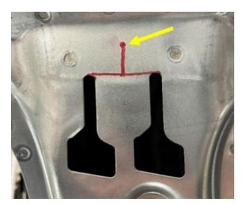
4. The top end of the vertical line, defines the exact position of the rework.
