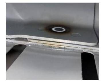
9. Clean and grind the welding surface to create a flat, smooth, and burr free surface. Then seal the entire area again with corrosion protection and paint.
