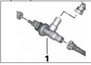
For the eligible vehicles and for the issue described below, BMW of North America, LLC (BMW NA) is extending the limited warranty for the vehicle's **Evaporative Emission Control** (EVAP) System's Purge Valve to:
