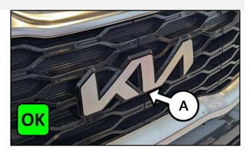
If the emblem (A) is not properly adhered to the front grille (or is found to be detached/missing) (NG); take a KVID video starting from the VIN label and show the partially adhered, detached, or missing emblem, and then proceed to the 'Replacement Procedure' below.
