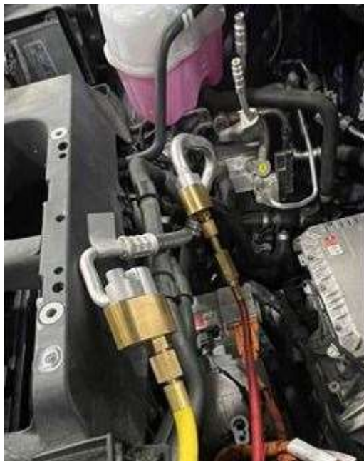
Figure 18. Installation of VAS 6338/3 and 6338/12.
