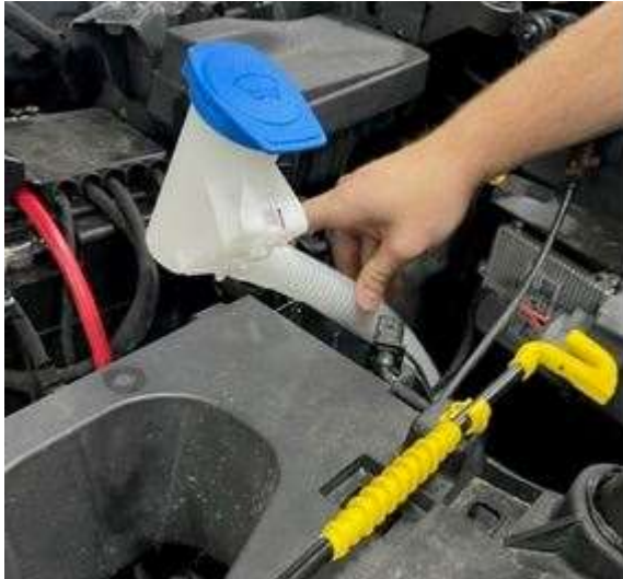
Figure 6. Set aside washer solvent filler neck.
