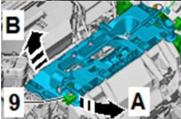
Figure 10. Lock carrier removal
