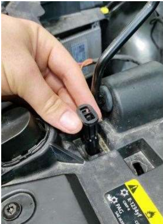
Figure 7. Remove radiator module bracket.
