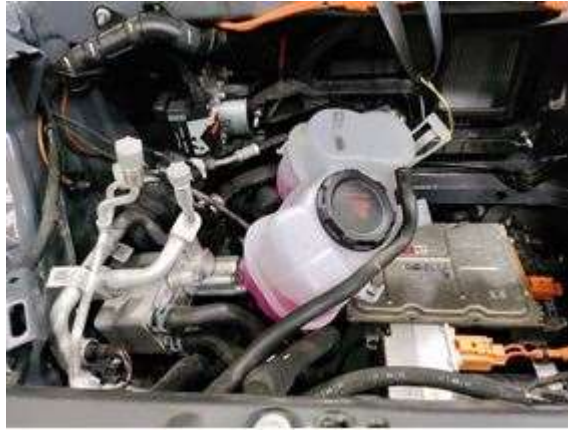
Figure 4. Coolant reservoir set aside.
