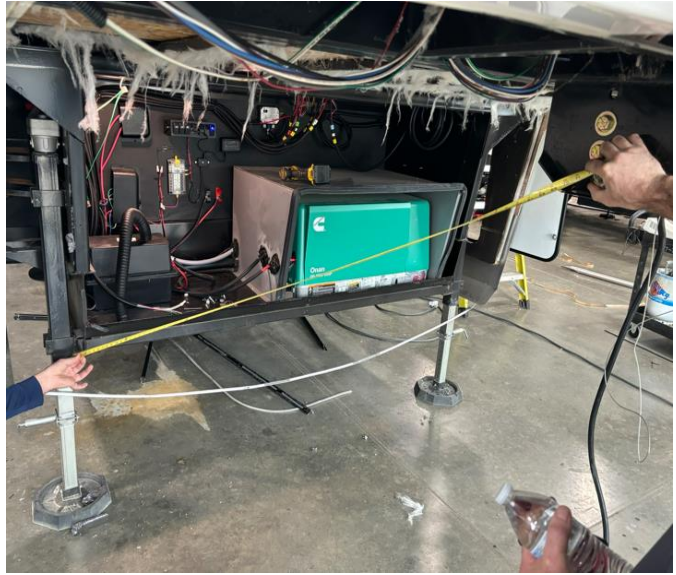
Example of measurement from I-beam to pin box
