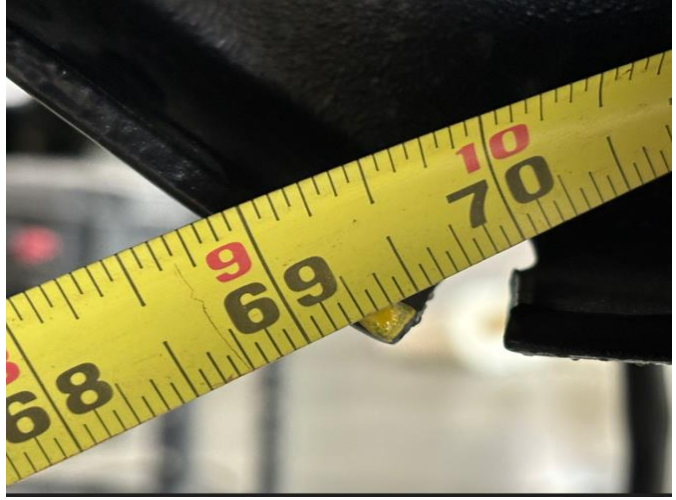
Example of measurement from I-beam to pin box
