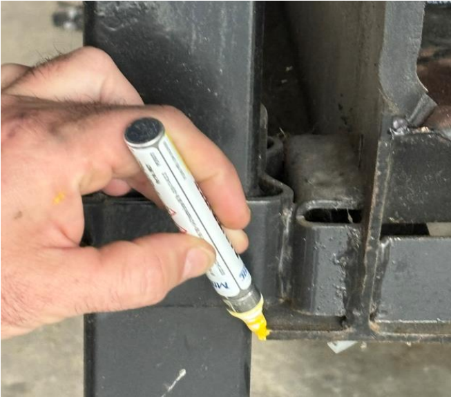
Example photo of index point on I-beam
