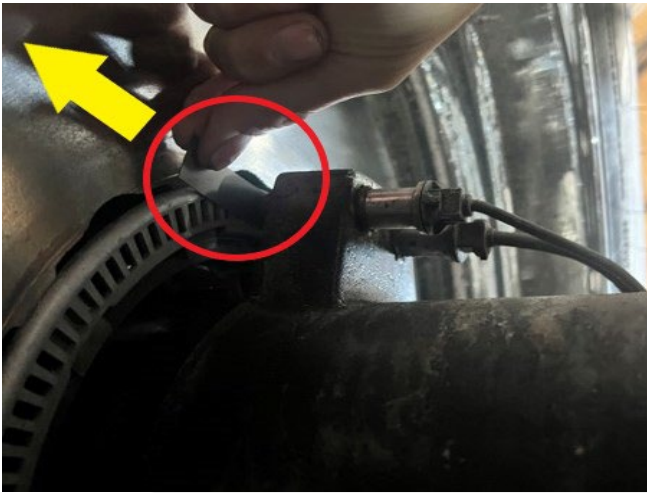
Figure 11 – Feeler gauge removal
