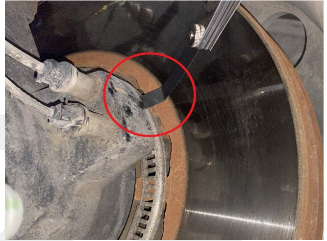
Figure 7 – Passive WSS and hub tone ring gap check
