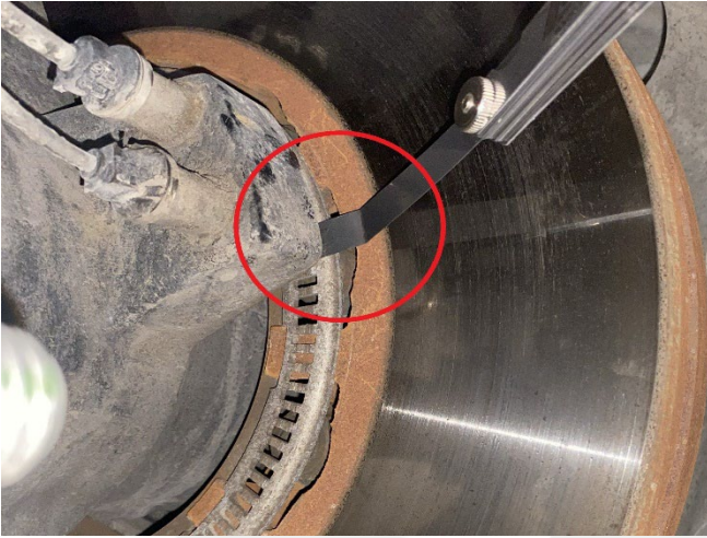
Figure 6 – Active WSS and hub tone ring gap check
