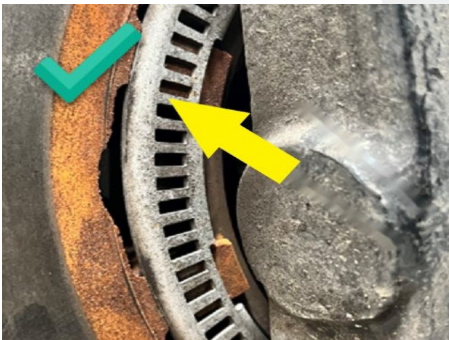
Figure 4 – Normal LH EDA hub tone ring wear
