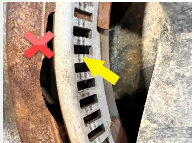
Figure 5 – Abnormal LH EDA hub tone ring wear
