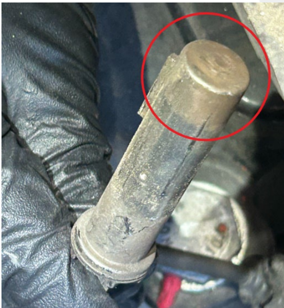
Figure 14 – Normal WSS wear
