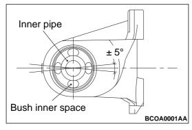
2. Assemble the bush so that the long protruding inner pipe is at the bottom of the vehicle and the bush inner space is in the position shown.
