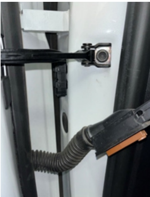
Figure 5 - Door Harness Connection Point
