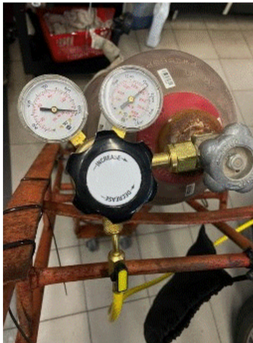
Figure 2. VAS 584005 pressure regulator attached to the calibration gas tank.
