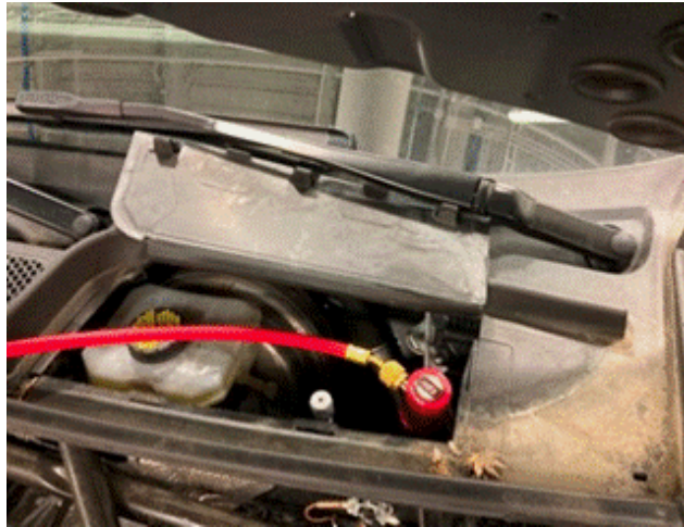
Figure 4. NITROKITG high side snap coupler connected to the high side service port.
