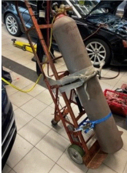
Figure 1. Calibration gas (95% Nitrogen / 5% Hydrogen).
