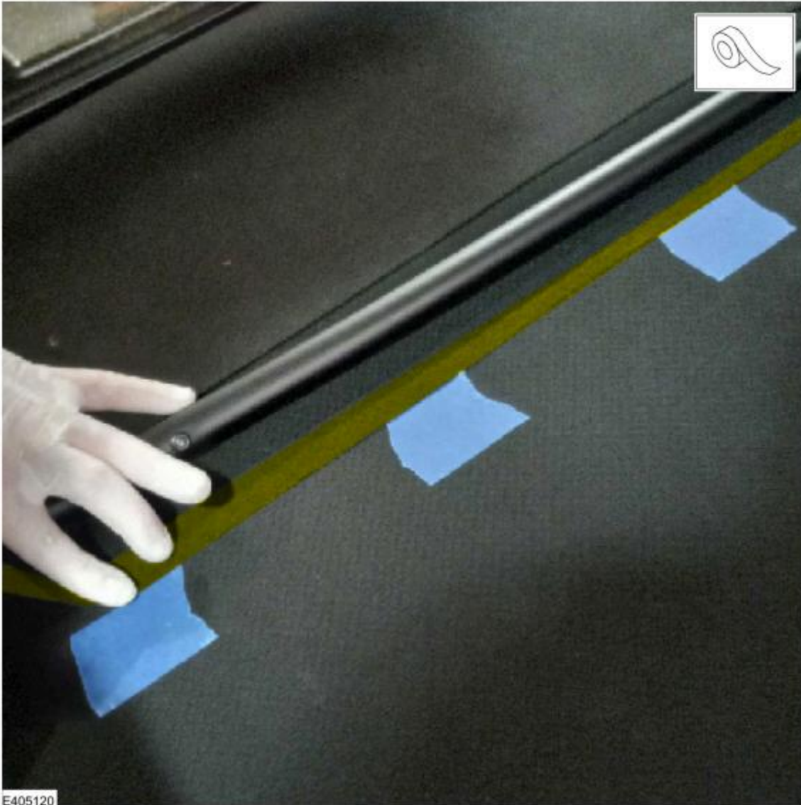
Figure 10 - Showing proper tape installation. Do not stretch tape and only remove backing as needed.
