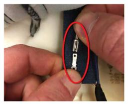
STEP 10: After connecting the new harness, place the new self-adhesive padding under the tail as shown (adhesive side up). Align the edge of the new padding with the two small, white registration marks on the tail as shown in (1) below. Peel the adhesive backing (2) and CAREFULLY apply the tail to the padding. Fold each side over (3) & (4) to recover it while being very careful to not create any wrinkles in the padding material.
