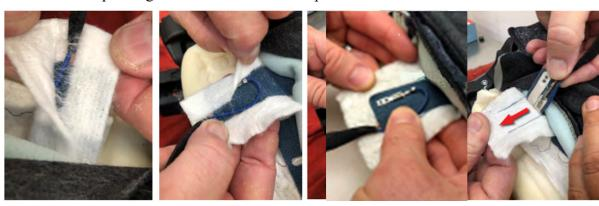
STEP 8: IMPORTANT: Before connecting the new harness, inspect the tail and sensor mat connectors to confirm they are tight on the 2 metal bands of the mat. Inspect closely for any breakages, cracks or other damages to the visible components of the sensor mat. If any damage is identified, the complete seat cushion assembly must be replaced as the sensor mat is not a serviceable component.
