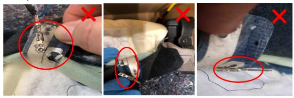
STEP 7: CAREFULLY peel the padding back to expose the tail and connections. Be advised, the adhesive used has a very strong grip. Hold the blue wire and CAREFULLY peel the padding in a direction parallel to the tail and discard. A new piece of self-adhesive fabric padding is included in the new replacement harness kit.
