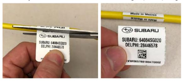
**STEP 12:** Remove the adhesive backing and apply the cut off section of the original label to the new replacement harness as shown in the photo sequence below.
