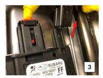
STEP 6: From the rear of the cushion (a cotter pin extractor works well), CAREFULLY release the plastic seat cover trim retainers as shown below and pull the back of the cover up as needed to access the harness to ODS sensor mat connection point (tail) circled below. The tail is covered in a self-adhesive fabric padding.
