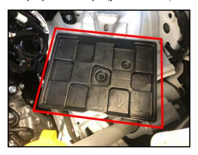
STEP 4: Install the replacement battery cover (p.n. 82123AN000) to the alternative replacement battery. Confirm the bottom of the cover is aligned flush with the bottom of the battery. DO NOT discard, this must be returned to the customer.
