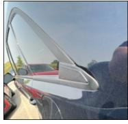
This is caused by the quarter window glass molding deforming due to harmful external conditions such as extreme heat or excessive force applied, and the double-sided tape fixing the molding's back side detaches. To eliminate this concern, the double-sided tape has been widened to enhance attachment.
