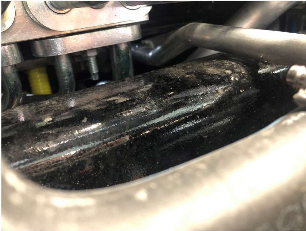
Fig. 1, Checking the Clearance between the Frame Rail and Coolant Pipe
