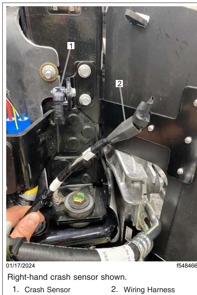
Fig. 4, Radiator-Mounted Crash Sensor
