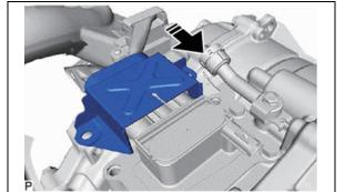
b) Slide the cover on the top side of the rear traction motor cable.
