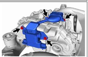
4. Remove the Rear Traction Motor Cable side mount bolts
