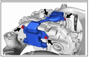
3. Install the 4 bolts for the rear traction motor cable.
