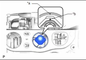
c) After tightening bolt (B), make sure the inner cylinder mark (a) and rubber part mark (b) are positioned as shown.
