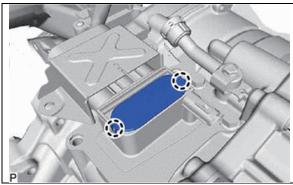
c) Disengage the 2 claws to remove the motor cable terminal cap from the rear traction motor with transaxle assembly.
