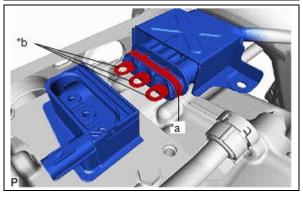
b) Remove Rear Traction Motor Cable from MGR Assembly.
