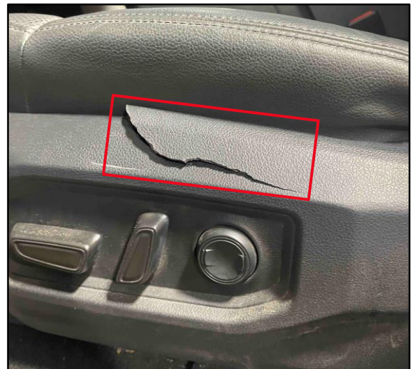
Figure 3. Broken Side-cushion Shield (8 WP)
