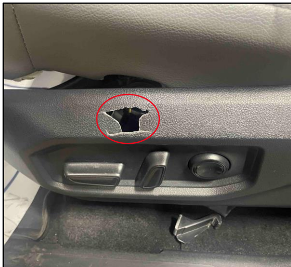
Figure 2. Loose/Broken Side-cushion Shield (8 WP)
