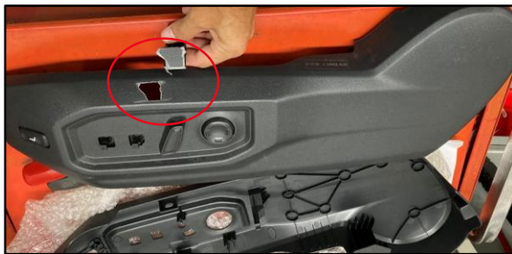
Figure 4. Broken Side-shield Cushion (10 WP)
