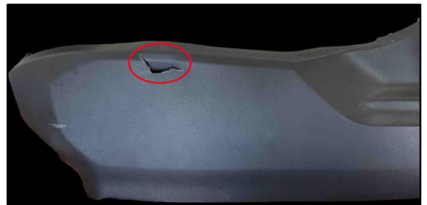
Figure 5. Broken Side-shield Cushion (4 WM)
