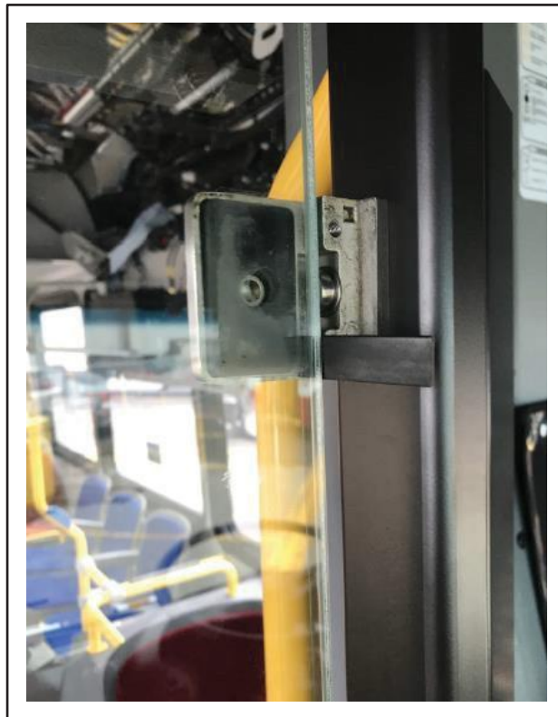
Figure 4 - Ensure 3 mm Gap on Side mounts
