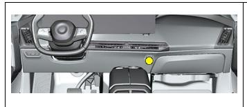
**NO**: If there is a customer concern for this situation **AND** the I-Level was newer than 22-11-540, only then replace the interior temperature sensor (B857, general location shown).
