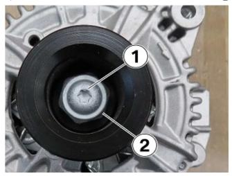
Check the retaining screw (1) for the hexagon nut (2) on the SGR drive pulley.
