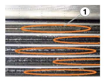
• Example: Belt debris in pulley grooves (1).
