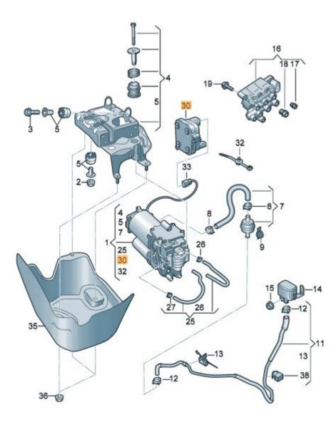
Figure 1. Verify that the compressor electronics is part number 4M0.907.778.A.
