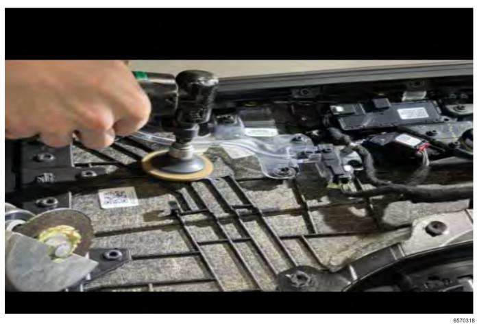
4. Then using a grind tool, smooth out the door panel.
