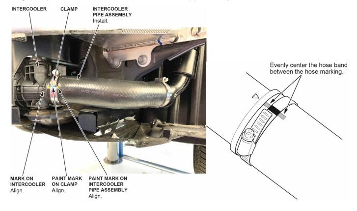
9. Tighten the hose bands to the specified condition below.
