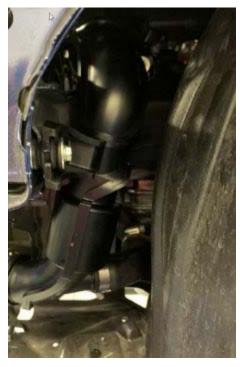
8. Slide the intercooler outlet hose onto the intercooler outlet pipe assembly. Then, install the hose band into position by lining up the paint mark, and the mark on the intercooler outlet pipe assembly.
