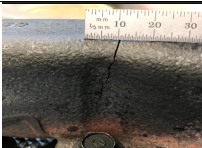
Fig. 2 Exhaust Manifold Crack
