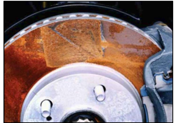
Figure 3. Severe Rust on Rotor (Hard to Remove by Braking)
