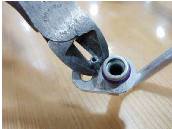
Figure 15. Removal of dowel pin.
