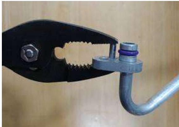
Figure 16. Installation of rear refrigerant line dowel pin.
