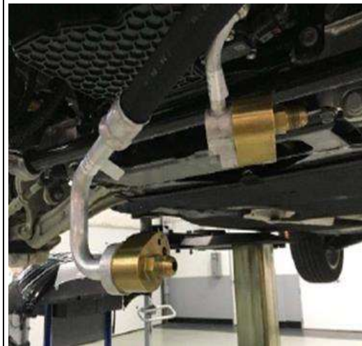
Figure 6. Installation of VAS 6338/3 and 6338/12.
