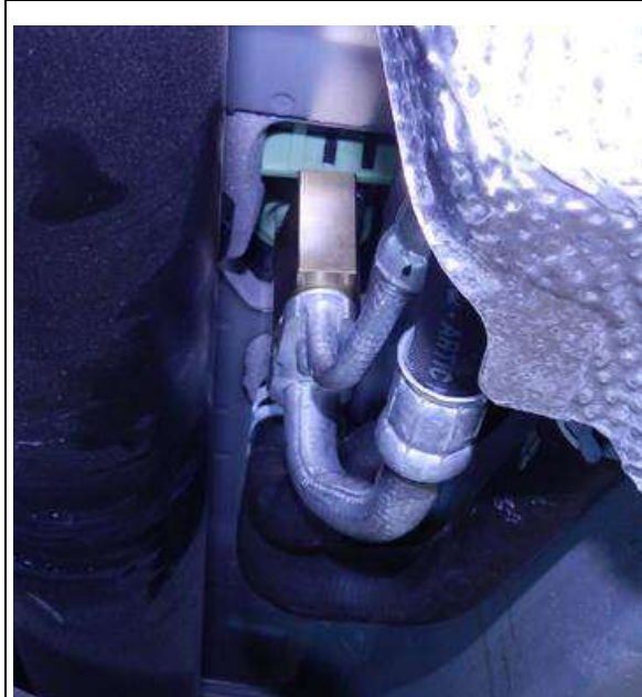
Figure 13. Location of rear air conditioning unit expansion valve.
