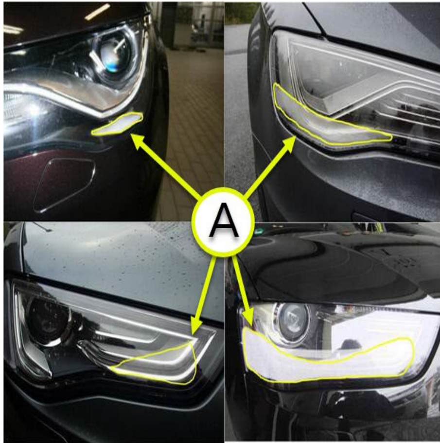
Figure 1. Normal condensation/moisture on the inside of the lights.
